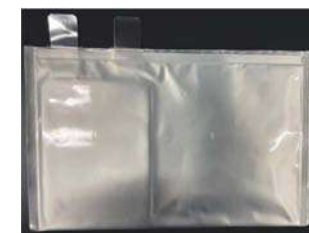
1.6 Ah Quasi-Solid-State Electrolyte Pouch Cell after Full Charging Puncture Test
